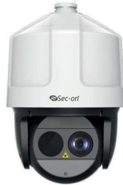
Laser smart PTZ Dome Cameras SC-SD2040-IR are able to capture high quality images in dim light environment with its laser IR light, which can reach up to 500m IR distance. Embedded with 1/3" progressive scan CMOS chip makes DWDR and 2MP real-time resolution possible. With the 30X optical zoom Day/Night lens, the camera offers more details over expansive areas.
